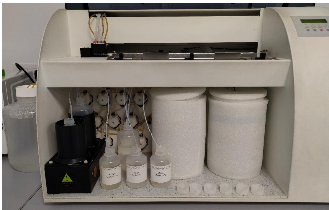
Figure 18. AutoLIPA robot from Innogenetics: There is a waste deposit, 6 dispensing tubes with distilled water bottles, two water tanks and the top part reserved for the tray with the nitrocellulose strips.
