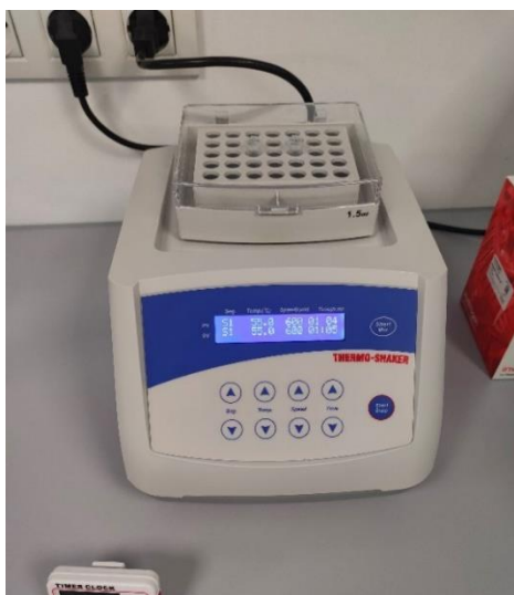
Figure 9. Thermo-block/Thermo-shaker: used to perform the incubation at 55 °C.
