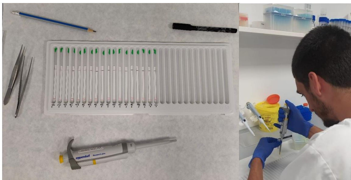
Figure 20. Hybridization method: On the left, the aspect of the tray with the different strips and their correspondent mixture of denaturant + PCR product (green color). On the right, me performing this step.
