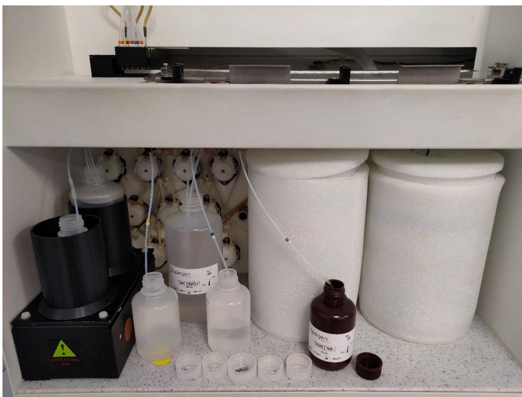
Figure 19. AutoLIPA dispensing tubes + reagents: Different dispensing tubes from AutoLIPA robot with their corresponding reagents.
